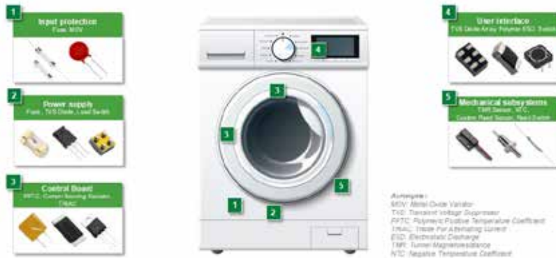
Figure 2. Components recommended for safe and efficient operation of a smart washing machine
